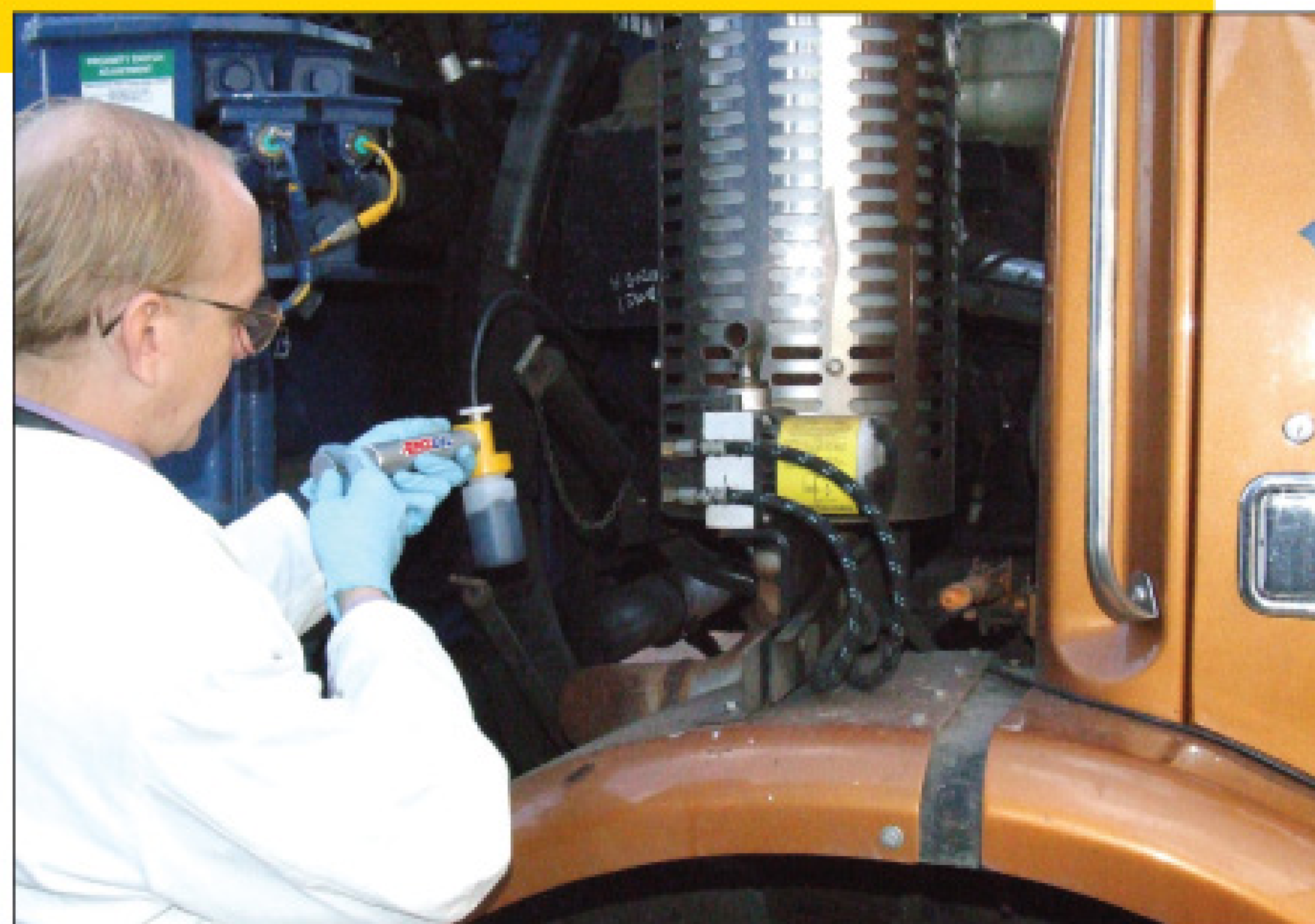
A technician draws an oil sample from a truck engine for analysis at a laboratory. Oil analysis is like a blood test for a machine — the results provide a picture of overall health and help diagnose trouble.
