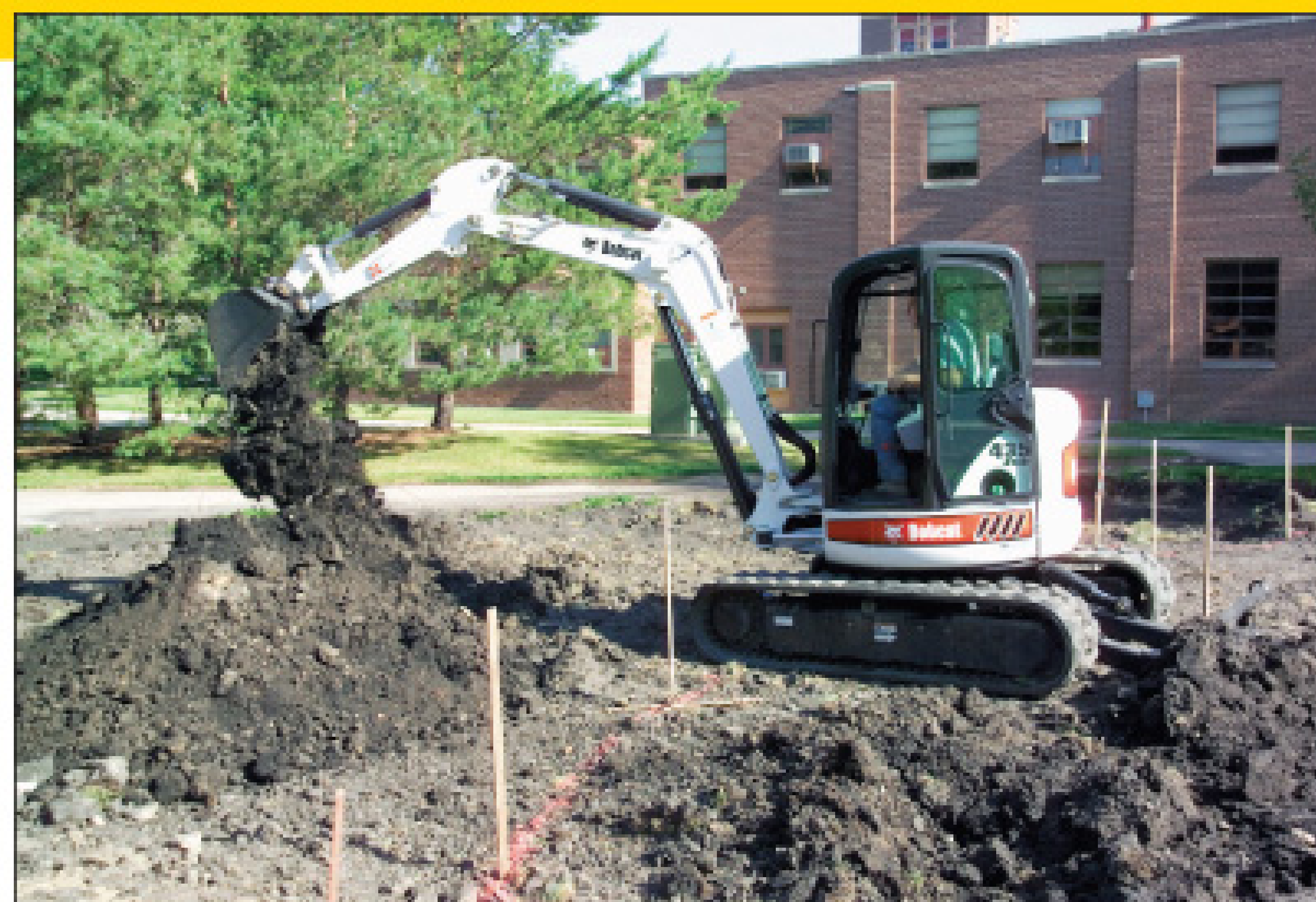
The Bobcat 435 zero-house-swing excavator has a shorter swing radius than a zero-tail-swing model.
