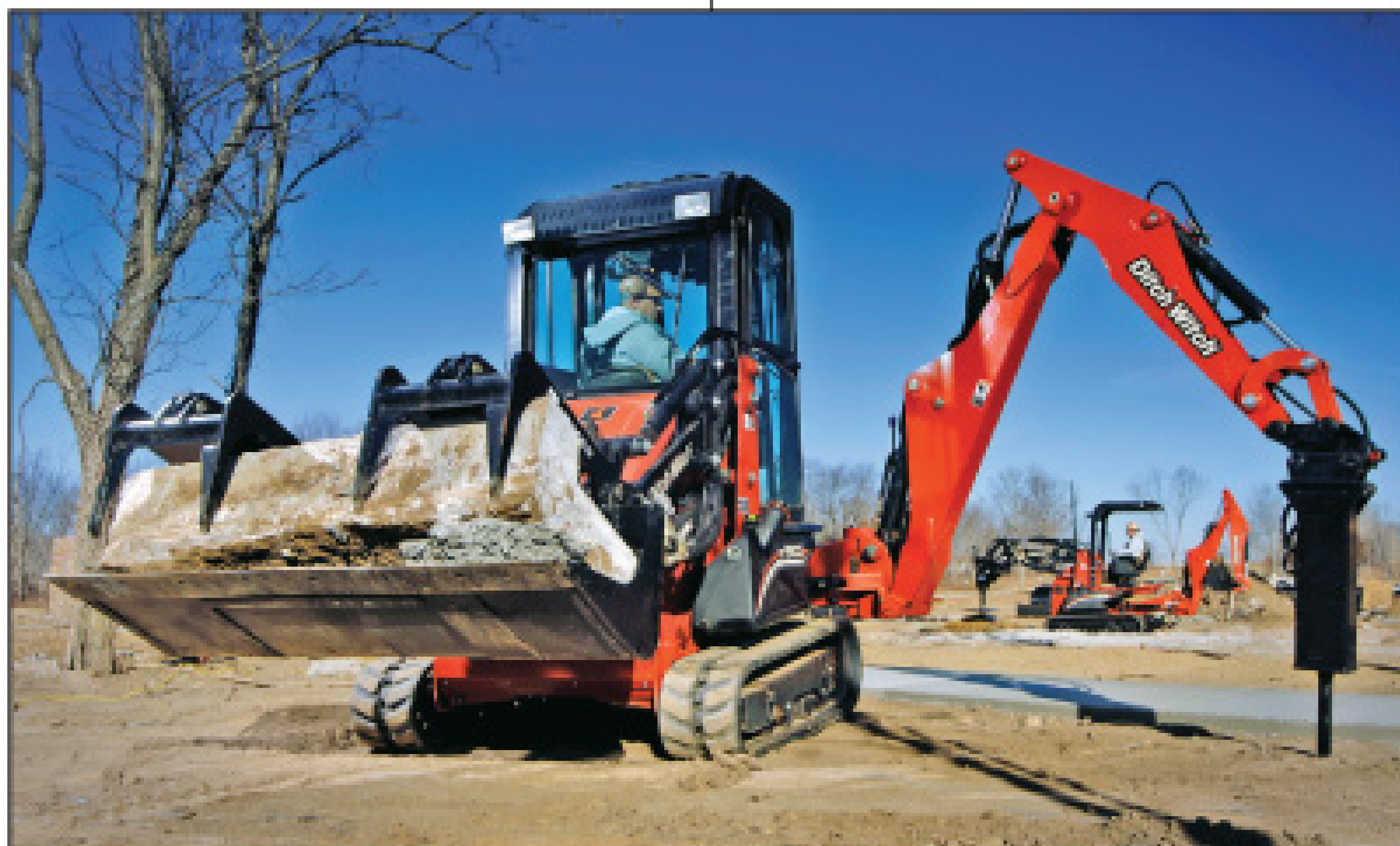
The Ditch Witch XT1600 rubber-track excavator-tool carrier combines attachment versatility with zero-radius turning.
