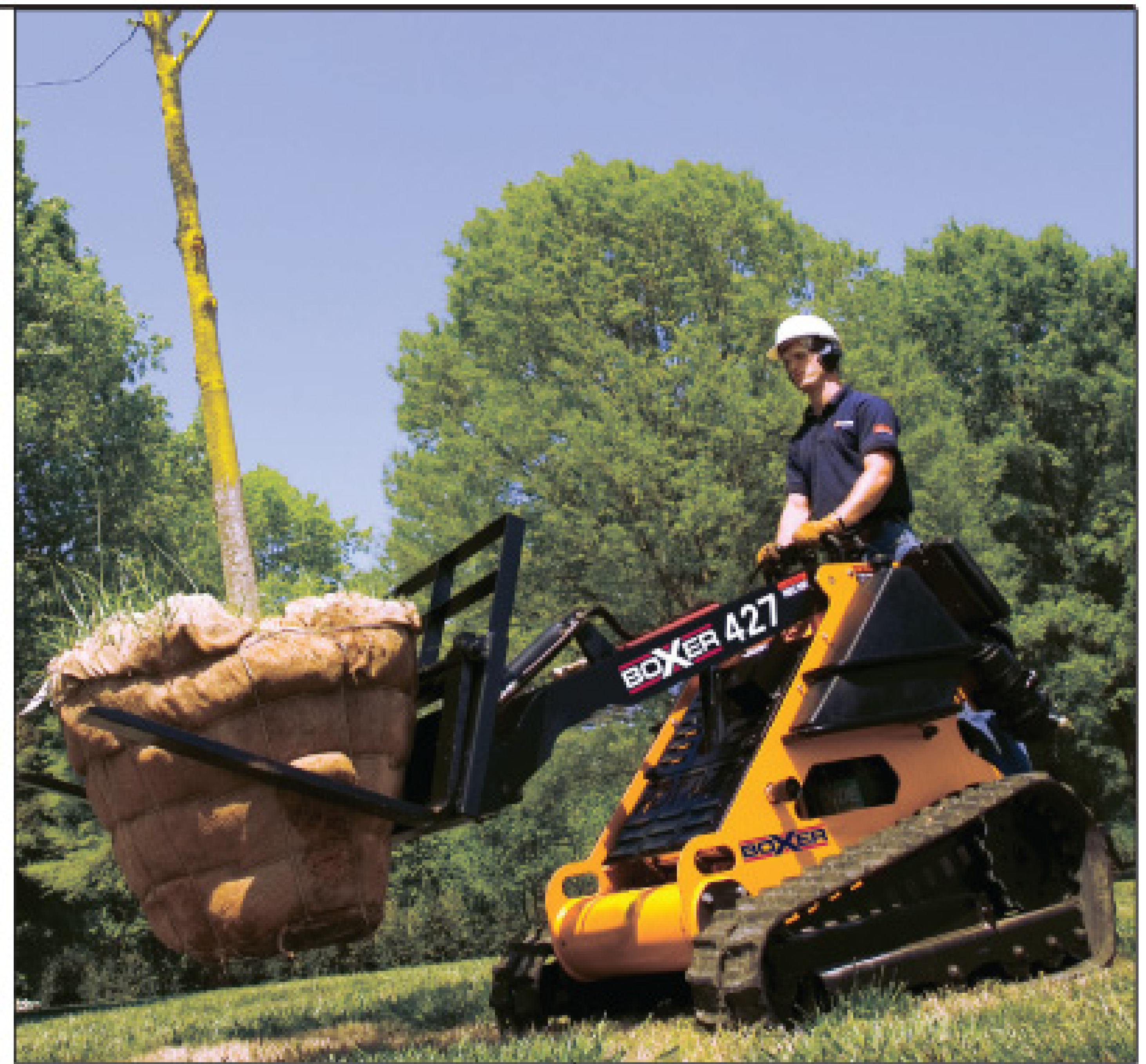
One advantage of a compact track loader like this Boxer 427 is its ability to lift more than a comparable size wheel loader.
