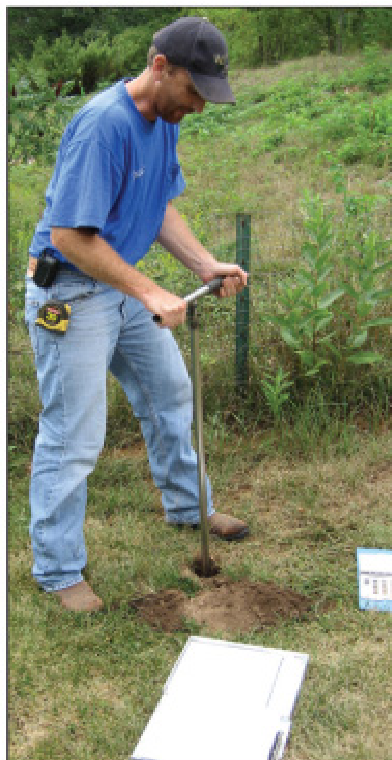
Tim Haig of Watab Enterprises evaluates the soil at the site using a 4-inch bucket auger. (Photos courtesy of Tim Haig and Watab Enterprises)
