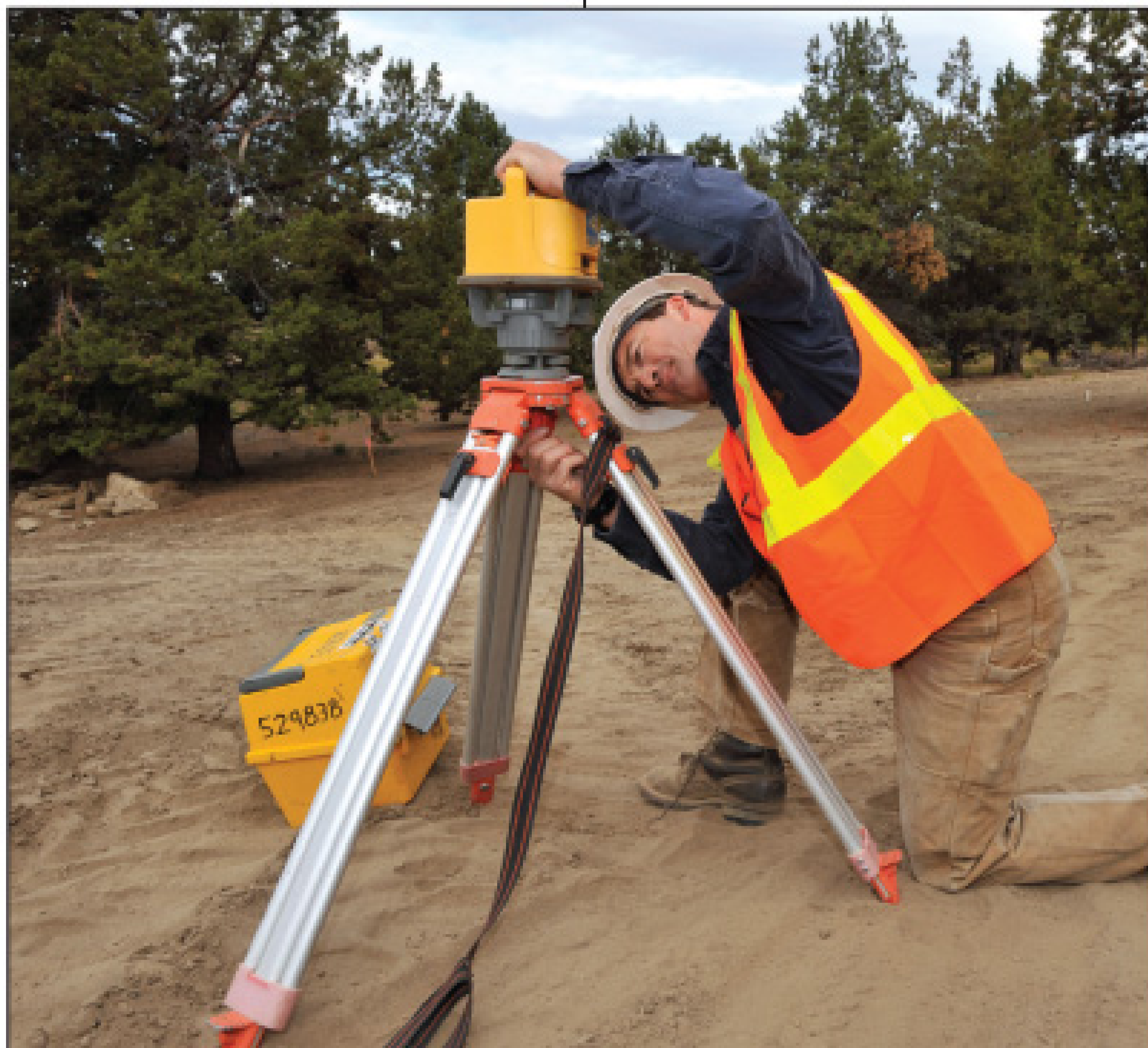
Brian Cyrus sets up a Spectra Precision Laser LL500 leveling system.
