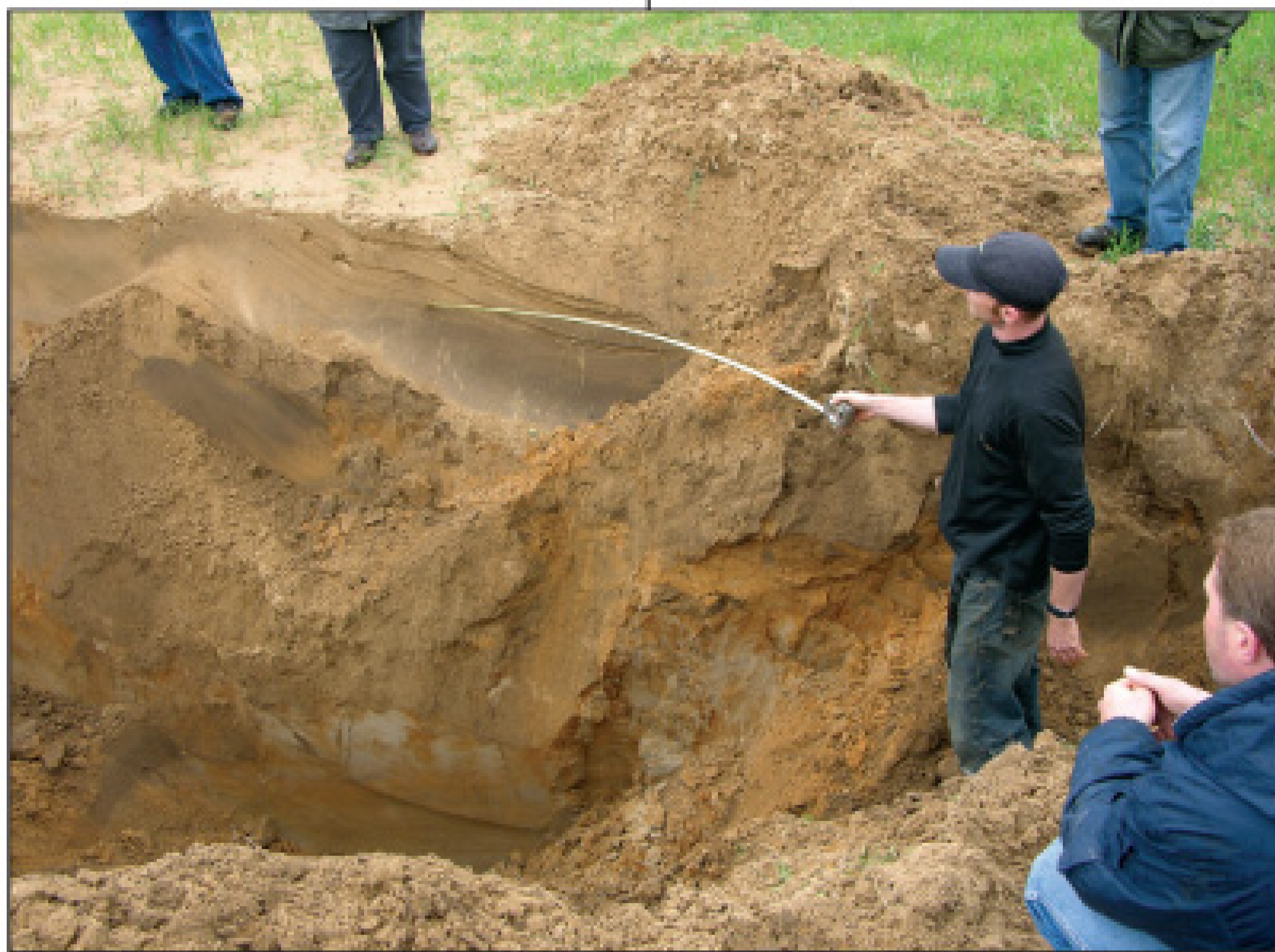
Soil Science instructor Dan Wheeler of the University of Minnesota points out color features in a soil test pit.
