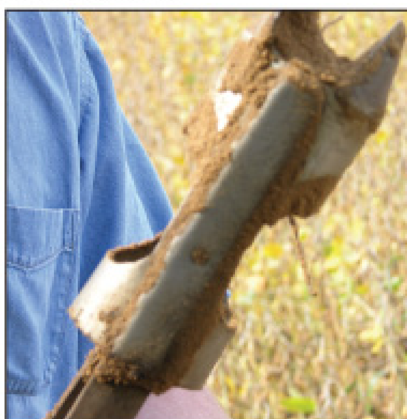
A three-inch-diameter bucket auger for soil borings.
