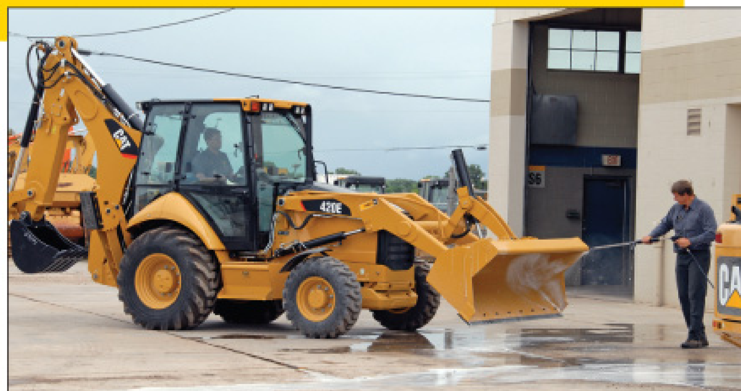
A thorough power washing will reveal issues you might need to address, says Dale Schraufnagel, of Schraufnagel Implement Inc., in Lomira, Wis. The photo shows a Cat 420E at FABCO Equipment Inc. in Green Bay, Wis. (Photography by Jim Kneiszel)
