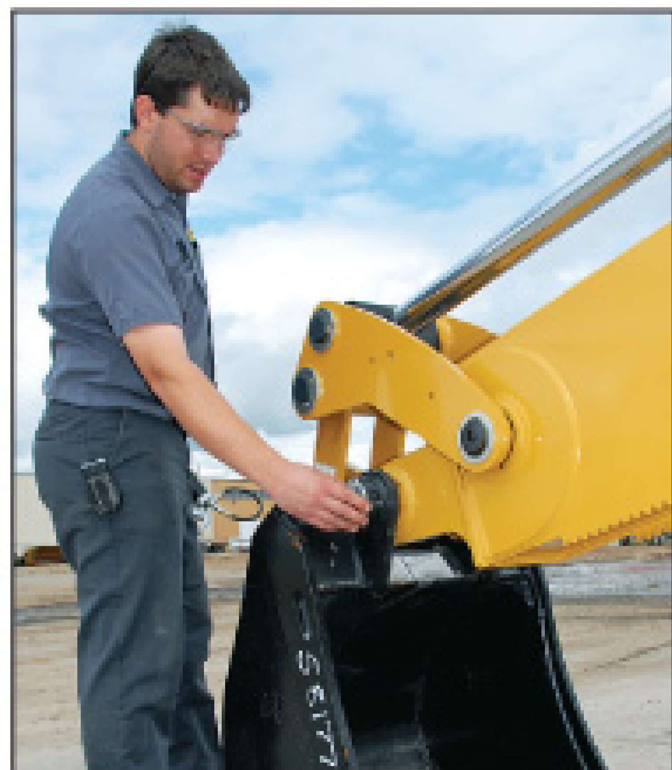
Inspect, clean and refresh all pivot points, bushings and bearings for smooth operation.
