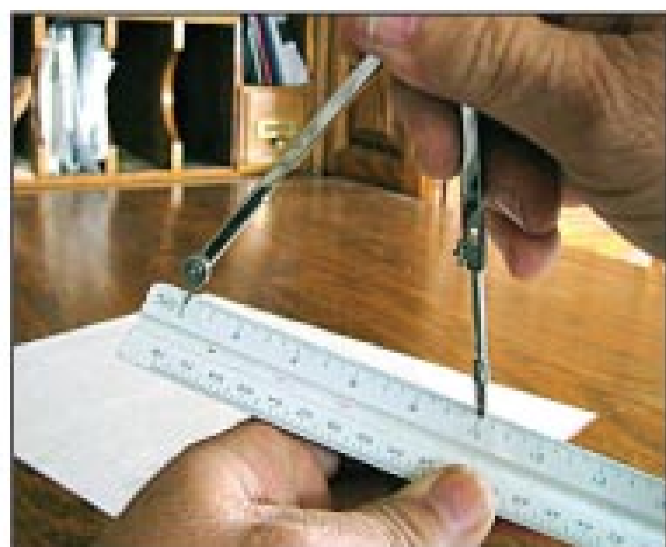
Creating good as-built drawings requires practice. Two useful tools are a compass and an engineer's ruler.
