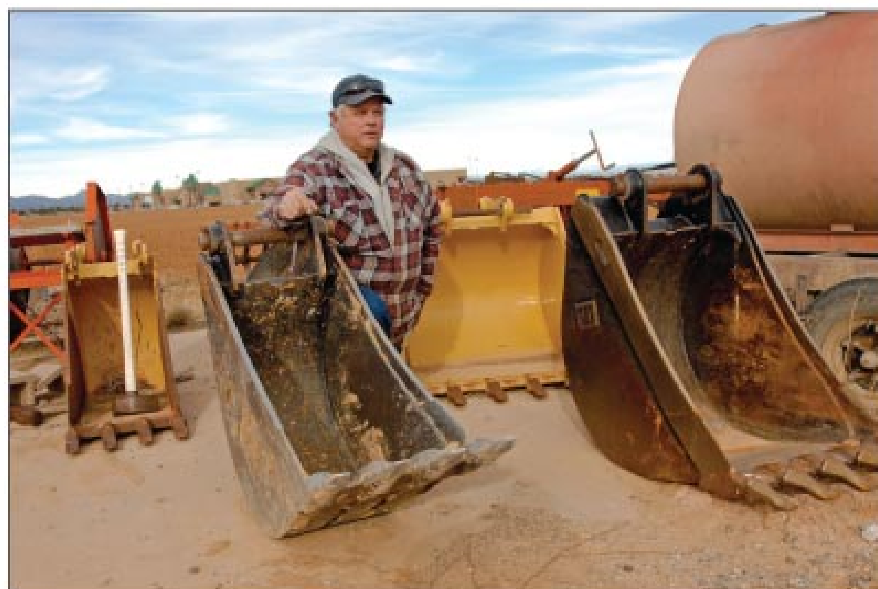
Bassett displays the various buckets he uses for digging trenches. He designs trenches from 18 inches wide (his personal minimum) to 36 inches (the regulatory maximum).
