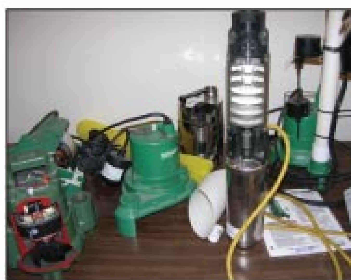
Onsite systems can use a variety of effluent pumps. The tall unit second from the right is a multistage pump.
