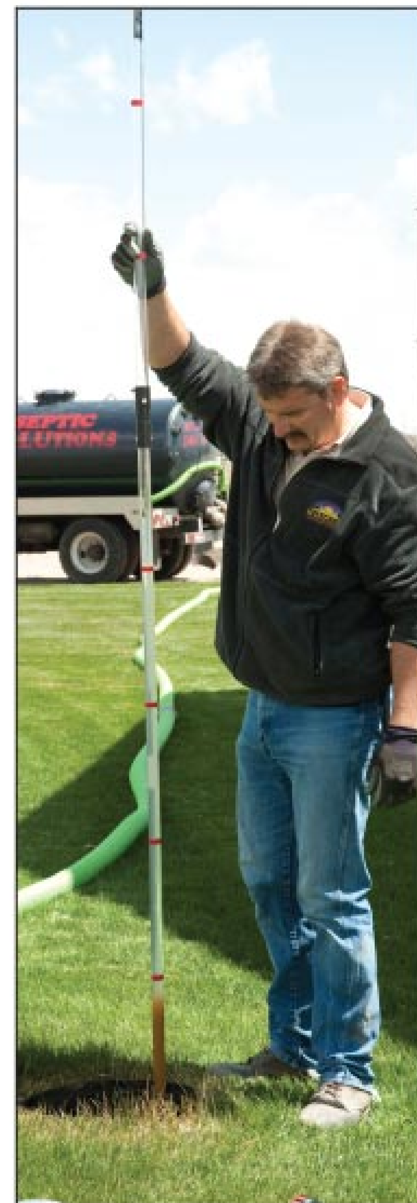
Kim Walker checks sludge thickness in a septic tank using a Sludge Judge from Nasco.
