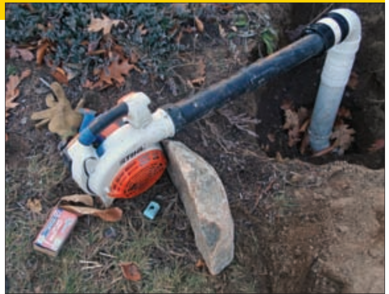
The test equipment: a handheld leaf blower connected to the inlet pipe of the septic tank, a rock to help deflect wind to help the smoke get into the blower, and a 30-second smoke bomb. (Photos courtesy of Russ Lanoie)
