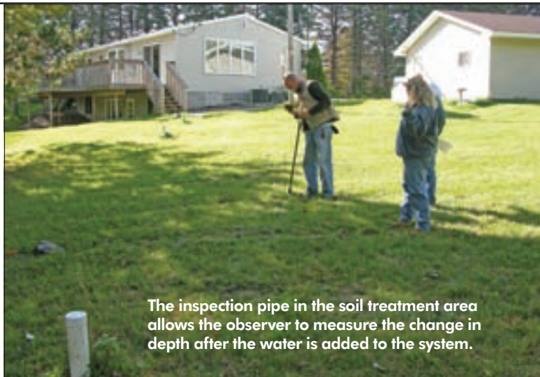
For the hydraulic load test, water is added through the septic tank. It is essential to know how much water has been added.
