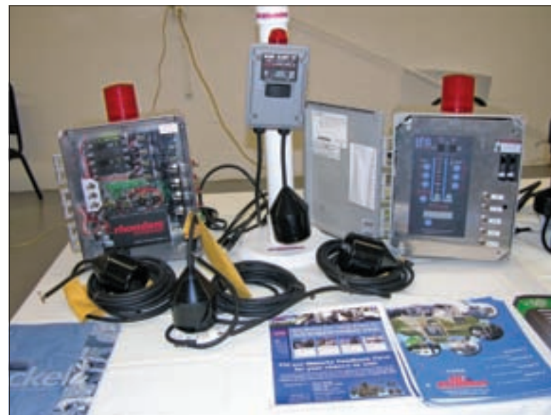
There are two ways to deliver effluent: through demand-dosing or by using a timer to control when the effluent is delivered to the next location in the system. Shown are systems from SJE-Rhombus.
