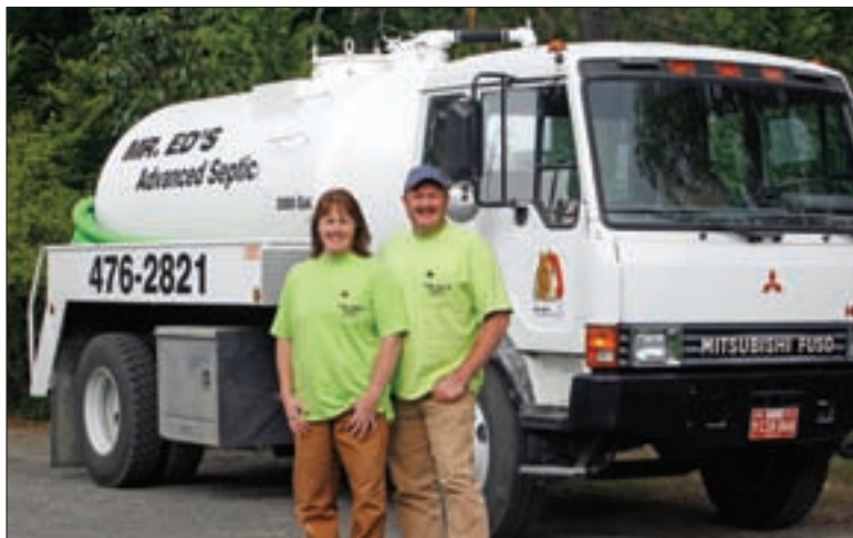
Stacy and Les Harris with the company's vacuum truck, a 1990 Mitsubishi Fuso HD-FX with a 2,000-gallon Leland tank and a Masport pump.
