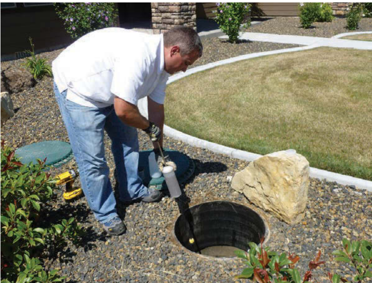
Ryan Spiers draws a sample of mixed liquor from the treatment tank.
