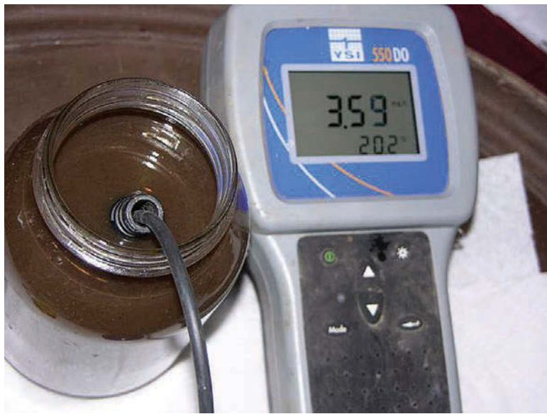
TOP: Here is a meter that can be used to measure dissolved oxygen in an aerobic treatment unit. LEFT: Two jars show the results of a basic settleability test.
