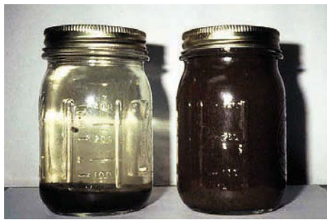
TOP: Here is a meter that can be used to measure dissolved oxygen in an aerobic treatment unit. LEFT: Two jars show the results of a basic settleability test.
