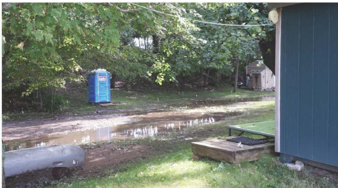
Look for site limitations, such as road easements and where excess water will collect, that can impact the viability of a proposed system.
