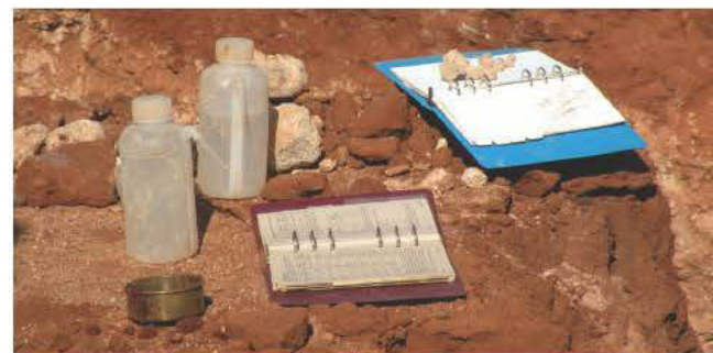
Some of the tools required for gathering soil information include a soil description manual, a soil color manual, a number 10 sieve and water bottles.
