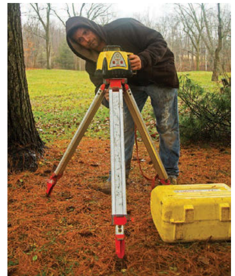
ABOVE: Baker lifts a 1,000-gallon Infiltrator Systems dosing tank during an install as Alberto Mendoza looks on. RIGHT: William Horgus sets up the Leica Rugby Pro 100 laser level to take a reading during a system install.
