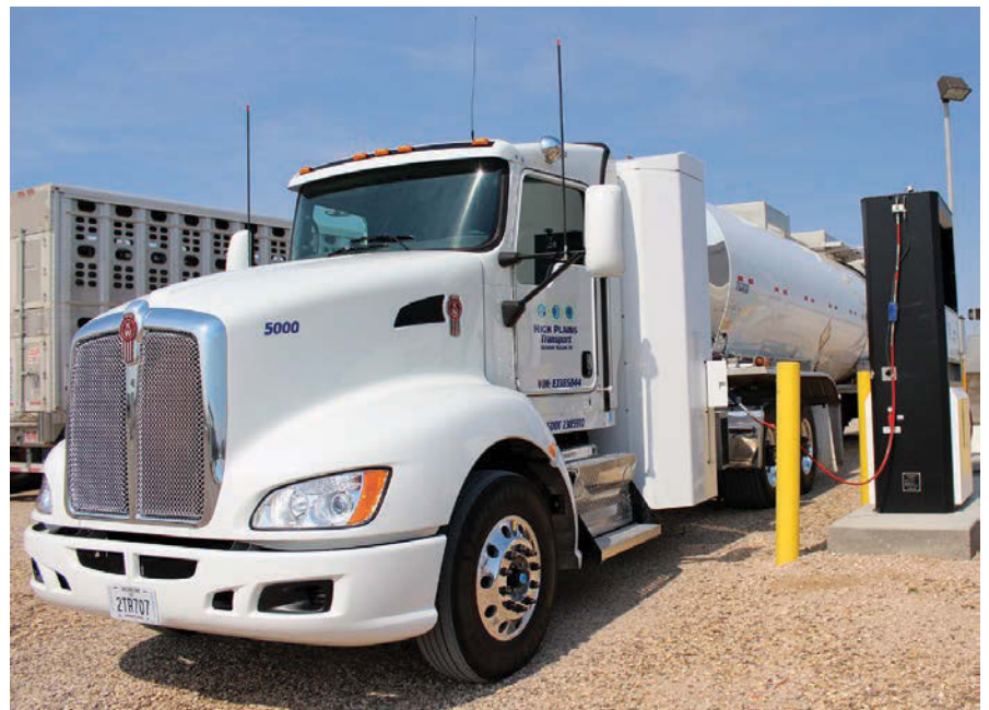
This High Plains Bioenergy rig is powered by a Kenworth T660 truck with Cummins Westport ISX12 G heavy-duty natural gas engine.
