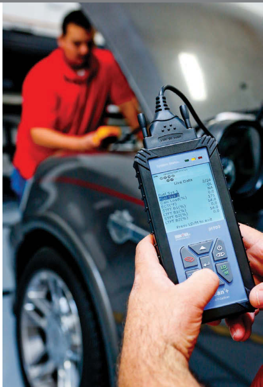
The Innova 31703 ScanTool at work diagnosing a problem in the garage. (Photo courtesy of Innova Electronics Corp.)
