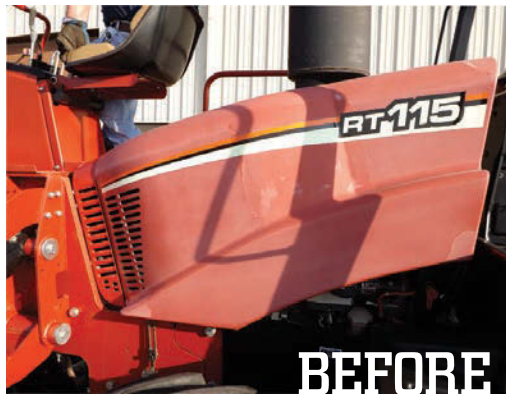
One of the best tips for maintaining a finish is simply to keep it clean. Ditch Witch offers Dakota Shine to restore faded surfaces, either steel or fiberglass, as shown in these before and after photos. Older equipment can be repainted and scratches should be touched up to prevent corrosion. (Photos courtesy Ditch Witch)
