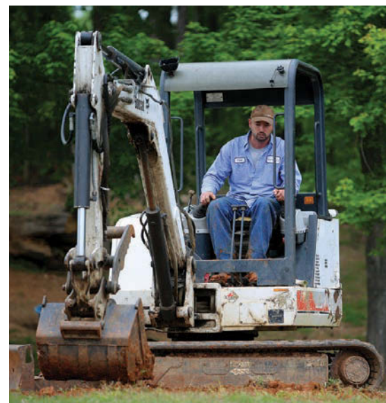
Brian Blake uses a Bobcat excavator to level ground after a septic tank installation.
