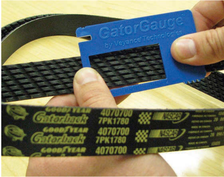
ABOVE: The GatorGauge tool offers three ways to inspect for belt wear. (Photo courtesy Veyance Technologies)
