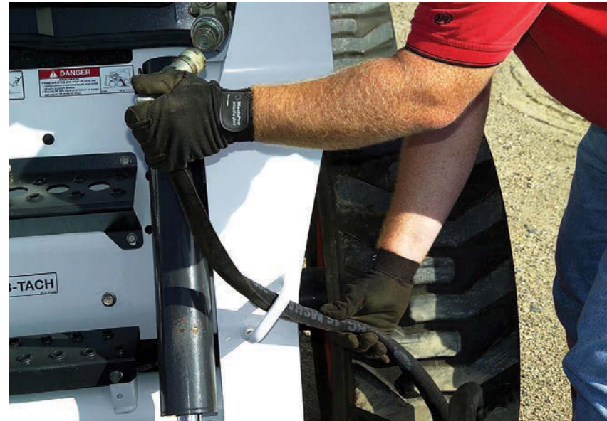
Dirt is the enemy of hydraulic fluid. Keep your system as clean as possible, particularly if using hydraulic couplers. (Photos courtesy of Bobcat)
