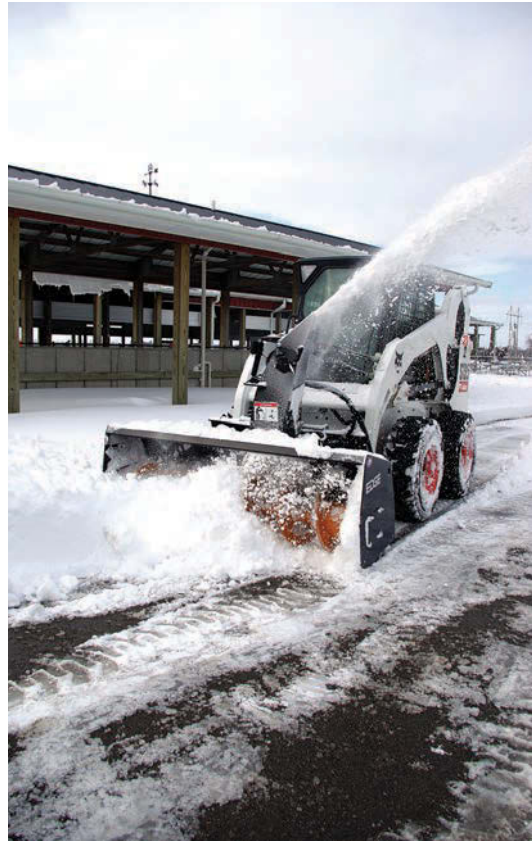
Snowblowers can be a handy winter attachment. Before sending yours out in the cold, be sure to check the hydraulic hoses for cracks and wear and the condition of the cutting edge and skid shoes. (Photo courtesy of CEAttachments)
