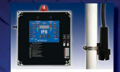
IFS Panels with C-Level<sup>™</sup> Sensor C-Level<sup>™</sup> sensor detects the liquid level in the tank and sends a signal to the IFS panel. Pump activation and alarm levels are adjusted on the panel touch pad, eliminating the need to go into the tank. One C-Level<sup>™</sup> sensor simulates up to four (float) levels.
