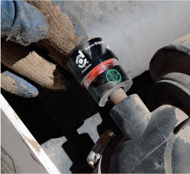
ABOVE: An air restriction indicator mounted to the air filter indicates when servicing is due.
