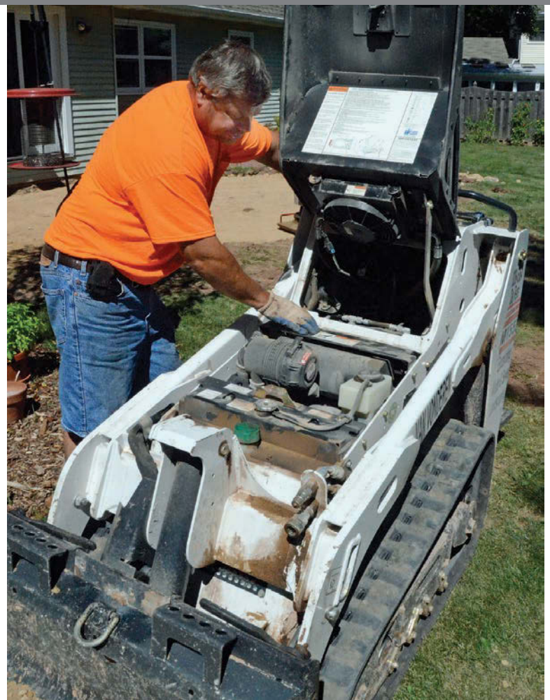
ABOVE: Steve Van Vonderen checks the engine oil, hydraulic fluid and radiator fluid each day. (Photo by Jim Kneiszel)
