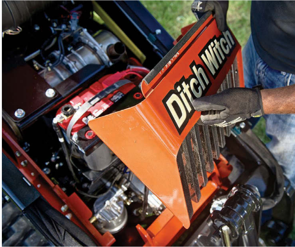
RIGHT: Ditch Witch recommends checking engine oil level, air filter service indicator, engine coolant level and hydraulic fluid level at startup and every 10 hours.
