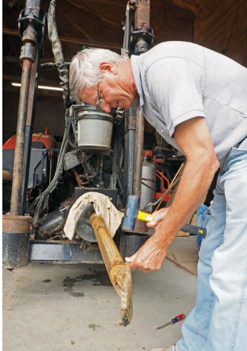
Billiet maintains the beacon assembly on his Ditch Witch JT2020 directional boring machine, a unit that has helped him expand the business into installation of geothermal loops.
