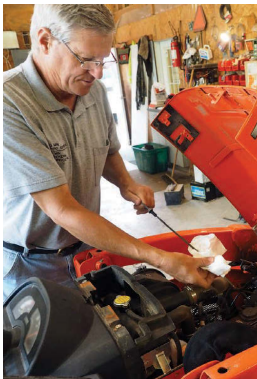
Bob Billiet checks the air filter and oil on his Kubota BX25 tractor/backhoe at the company shop before heading out to a work site.
