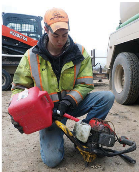
Technician Nick Simonsen fuels a Crust Buster tank agitator in the company yard.
