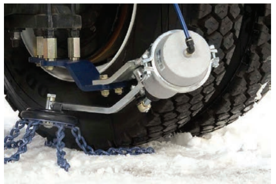
The Onspot automatic tire chain system provides on-demand grip when you hit snow and ice.
