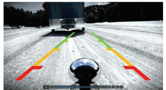
The Tow-Hitch Assist, an option on Ford Transit vans, enables one person to easily attach a trailer.
