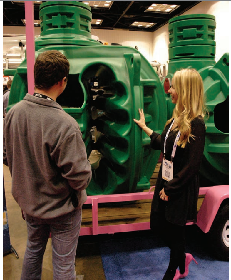
Annette Simon, right, marketing coordinator for Norweco, explains the added filtration benefits of the Hydro-Kinetic Bio-Film Reactor. The unit is added to existing treatment systems to produce cleaner, more consistent effluent. (Photo by Craig Mandli)
