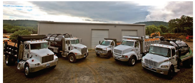
BELOW: The New Milford Septic fleet includes, from left, 2001 Peterbilt dump truck with a Beau-Roc body, a 2008 Peterbilt 340 with 3,250-gallon Presvac Systems steel tank and Challenger 367 pump, 2006 Chevy 5500 six-wheel dump truck with 5-cubic-yard Beau-Roc box, 1999 Sterling LT 9500 tri-axle dump truck with 18-cubic-yard Beau-Roc box, and a 2006 Freightliner M2-106 with 2,600-gallon Imperial Industries steel tank and Jurop/Chandler pump.
