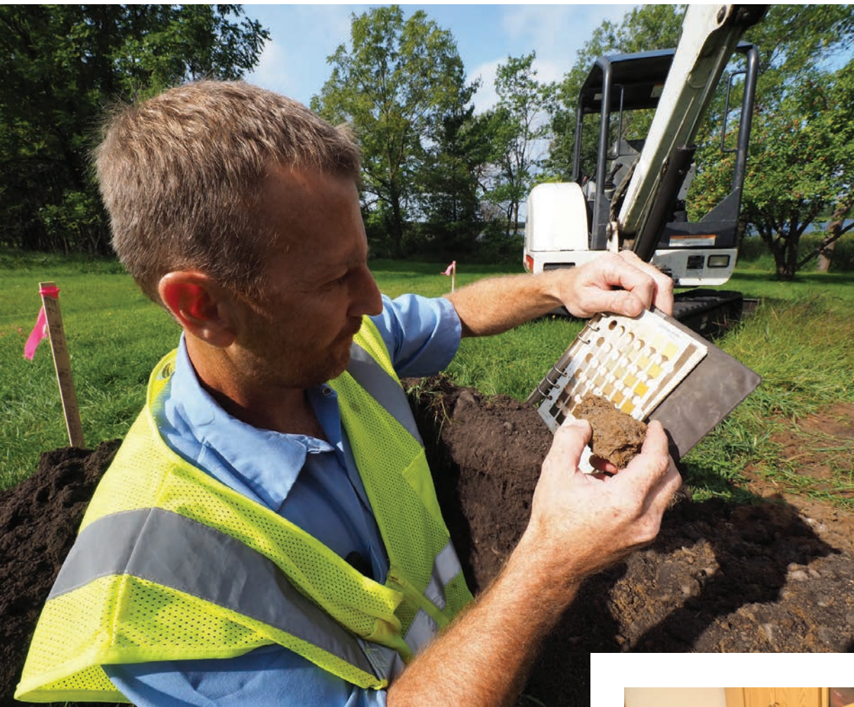
<<LEFT: Tim Haeg performs a site evaluation comparing soil samples in a test pit with a Munsell color chart. A Watab Inc. Bobcat 331 mini-excavator is shown in the background.
