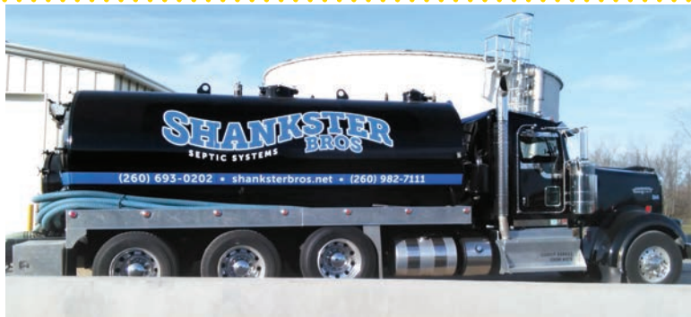
▲ Steven Shankster's big rig is a 2015 Kenworth W900 with a 4,800-gallon tank and Masport pump built out by Morocco Welding.
