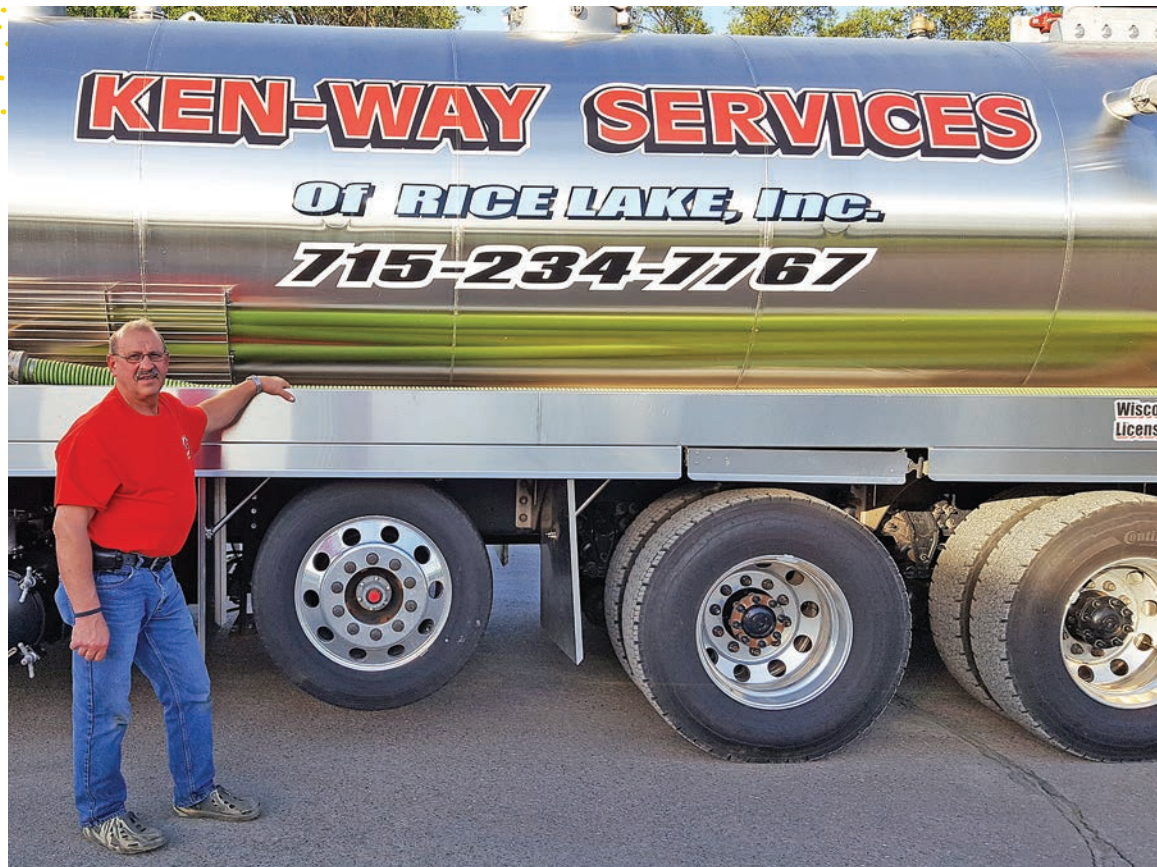
▲ John Bowen and 2017 International with an Advance Pump & Equipment 4,300-gallon stainless steel tank and Wittig (Gardner Denver) pump.
