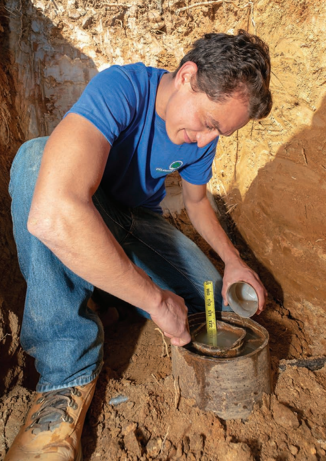
◀◀ Nestor Barillas Anaya performs a perc test at a system installation site. (Photo by Kevin Blackburn)
