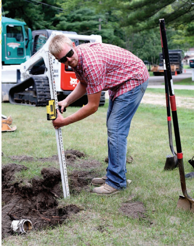
◀ Zach Rodriguez uses a Leica Rugby 680 laser level system on a job site.
