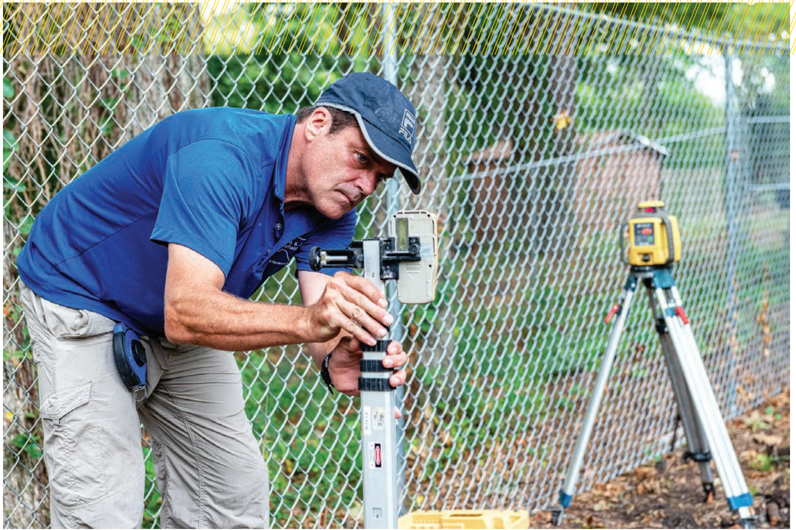
▲ Ric Seley measures the depth of an excavation using a Topcon laser level.
