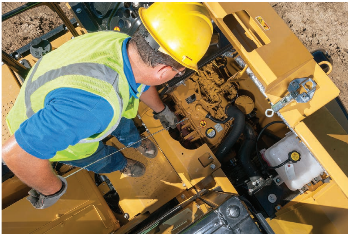
A contractor performs engine maintenance on a Caterpillar excavator. The oil and grease checks should be completed on a regular routine. (Photo courtesy of Caterpillar)
