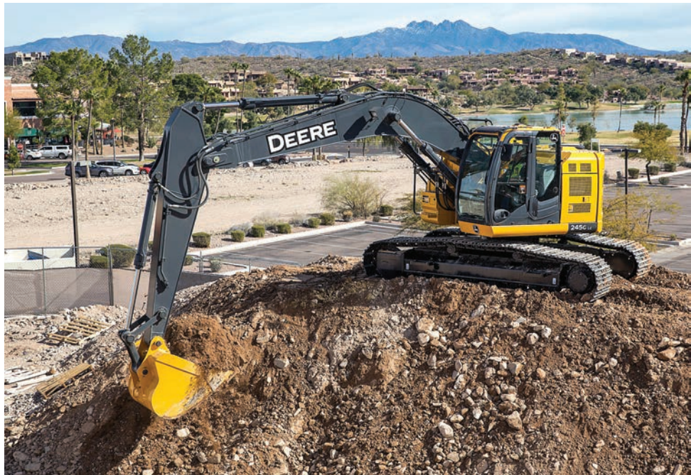
Keeping the bucket teeth of an excavator sharp will help keep the equipment productive for a contractor. (Photo courtesy of John Deere)
