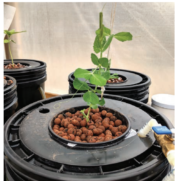
▲ To treat wastewater, the Massachusetts Alternative Septic System Test Center built several sand columns using these large plastic drums. Brian Baumgaertel, the center’s director, is a fan of sand columns because they do a good job of treatment at low cost. Plants were set on top of the columns so their roots could feed directly on the water inside.
