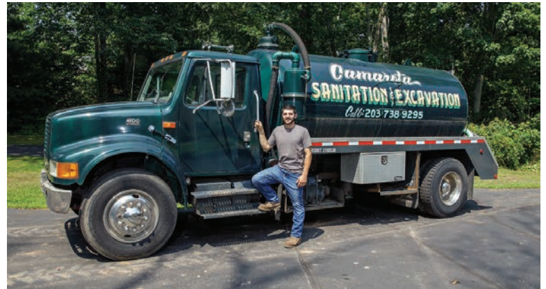
▲ Camarota broke into the wastewater business with a 2000 International 4900 with a 2,500-gallon steel tank and Jurop pump that still serves his installing business.
