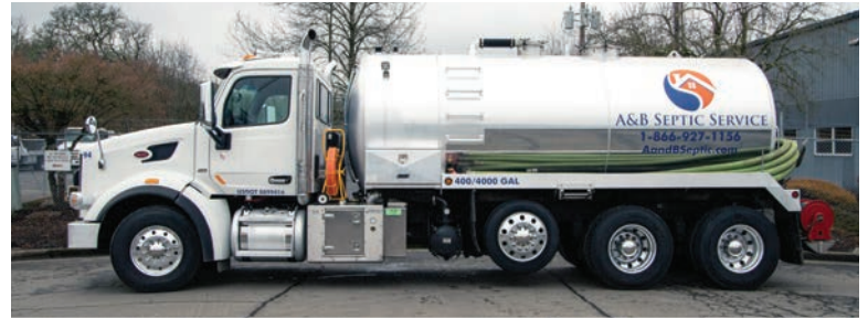
▲ A&B Septic Service runs this 2021 Peterbilt 567 built out by Imperial Industries with a 4,200-gallon stainless steel tank and National Vacuum Equipment pump.
