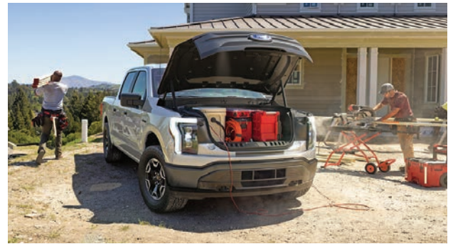
▲ Without an engine up front, EV trucks convert that space into a "frunk" or front trunk — secure, weather-tight spaces. In the Ford Lightning, the space is large and includes a variety of outlets to power tools in the field.
