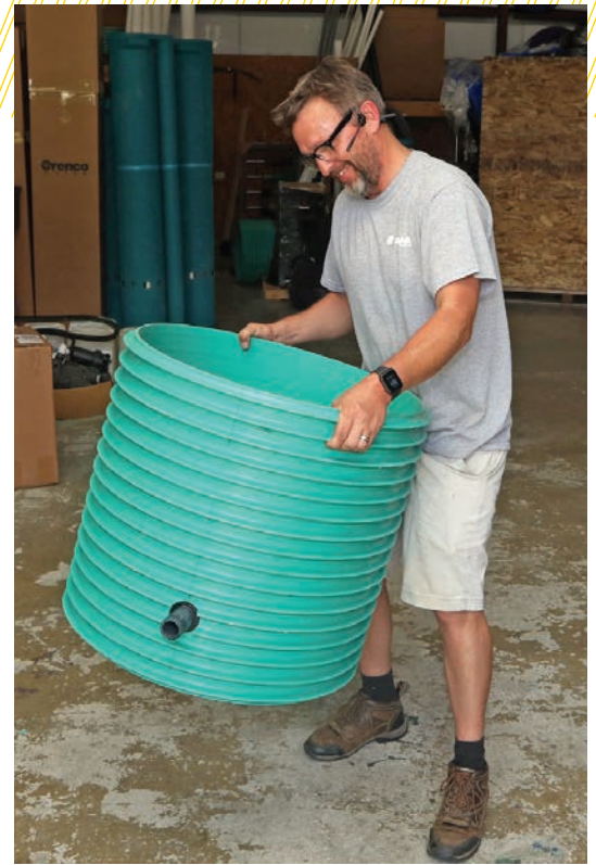
▲ Kevin Johnson assembles an AQWASTEP street connection used in conjunction with an Orenco Biotube ProPak pump package.
