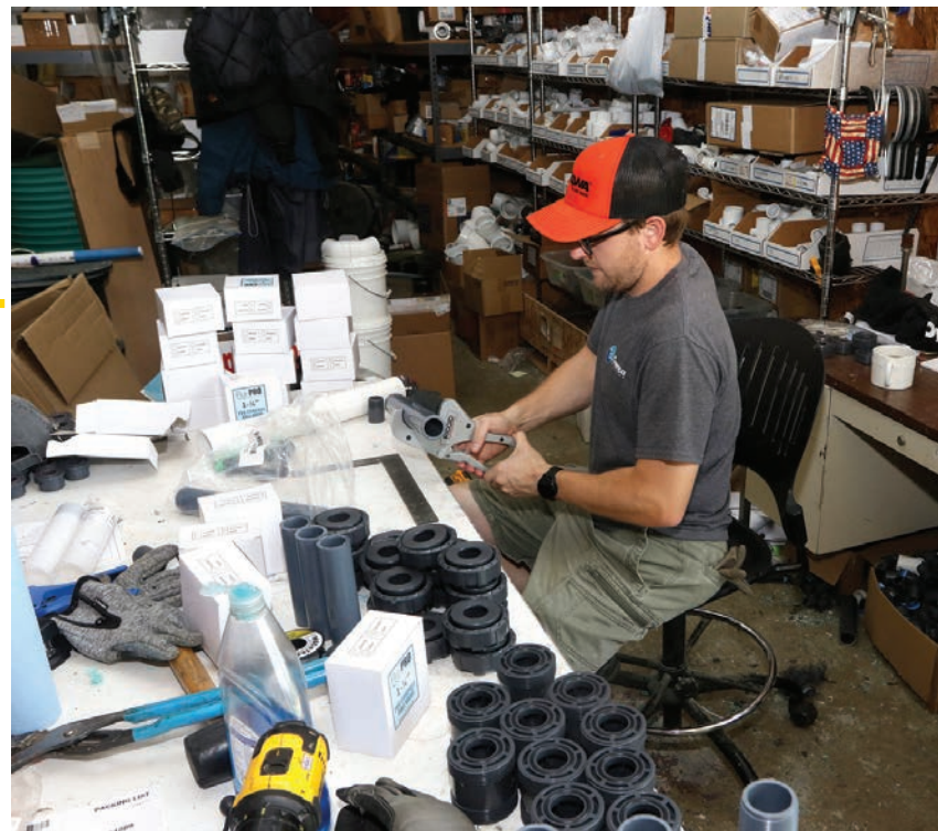
▶▶ In the company shop, Stuart Webb assembles valves used in the Orenco Biotube ProPak pump package. AQWA provides tank adapters, lids and risers for STEP systems.
