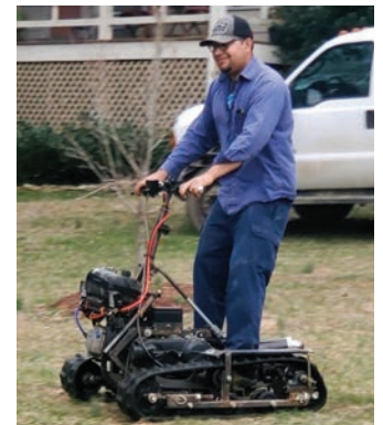
▲ Valentino Garcia and the "Track Buddy" he designed and built to quickly move around a job site.
