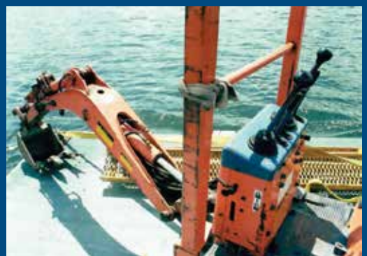
▼ The 1,800-pound KH007 compact excavator (Kubota) is parked precisely in the center of the 12-by-12-foot powered wooden dock.
