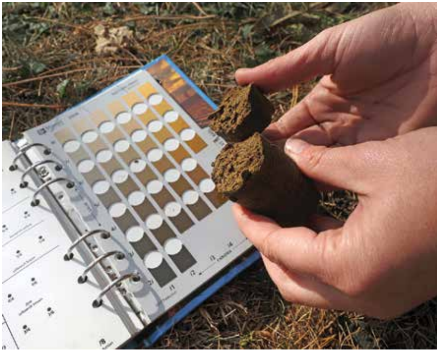
◀ Stacey Feser checks a core sample for a system installation, consulting with the Munsell Soil Color Book.
