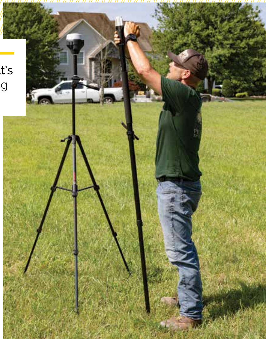
Adam Browning sets up Emlid surveying equipment during a site evaluation for a new onsite system.
